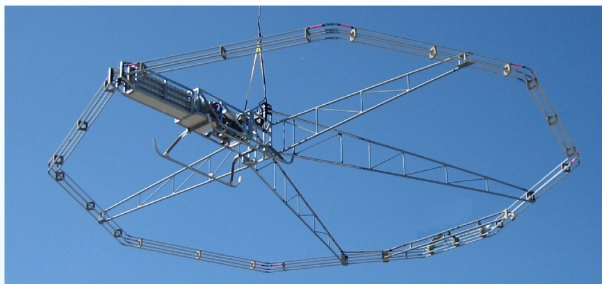
The THEM transmitter airfoil, total towed weight less than 300 kg
