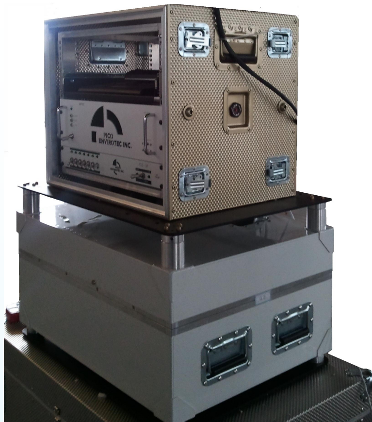
Pico Envirotec's AGRS airborne gamma-ray spectrometer system. This system includes 16.8 litres of NaI(Tl) detector downward-looking and 4.2 litres of detector upward-looking. Also shown is the equipment rack, which contains an IMPAC data acquisition system and GPS receiver.
