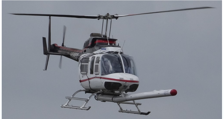
HELIMAG system, featuring one cesium vapour magnetometer measuring the total magnetic intensity, installed on a Bell 206L3 Long Ranger Helicopter
