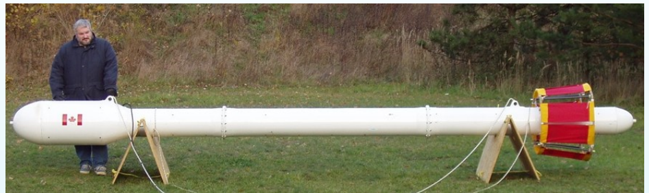
HUMMINGBIRD 5-frequency sensor, 7.5 meters long in 3-sections, 30 metres long tow-cable
