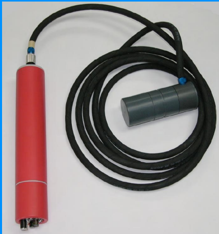
Scintrex CS-3 cesium vapour magnetometer, sensitivity of 0.001 nT sampling at 10 or 20 Hz.
