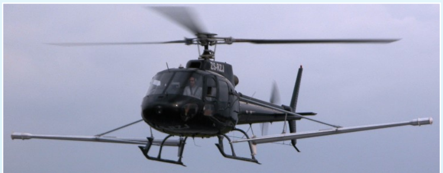
HELIGRAD system, featuring two cesium vapour magnetometers measuring the horizontal gradient of the magnetic field as well as the total magnetic intensity, installed on a Eurocopter AS350B2 Helicopter
